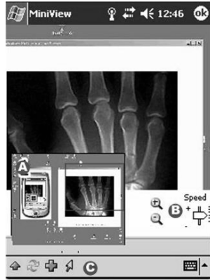
Fig. 2. Proximity-based application sharing functionality (a) The MiniView tool provides a small depiction of the information shared (b) The directional pad used to control de speed of the cursor (c) Options of the application sharing application
